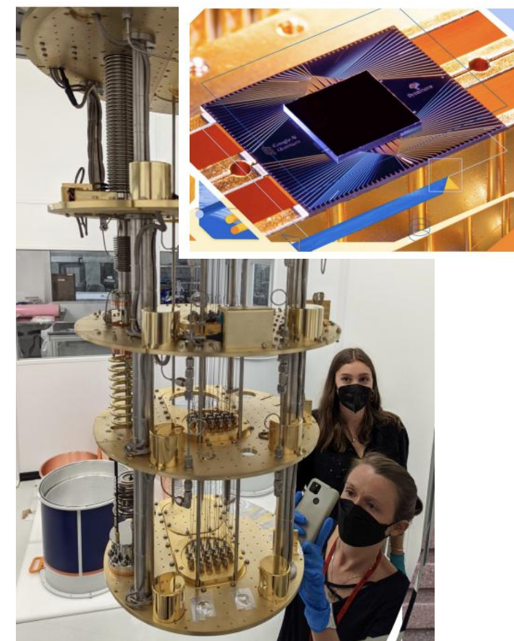
Test stand for quantum detectors • Can go below electron energy threshold
